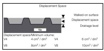
The displacement space (v4-v10) is the open space between the upper walked-on surface and the drainage level of profiled surfaces.
