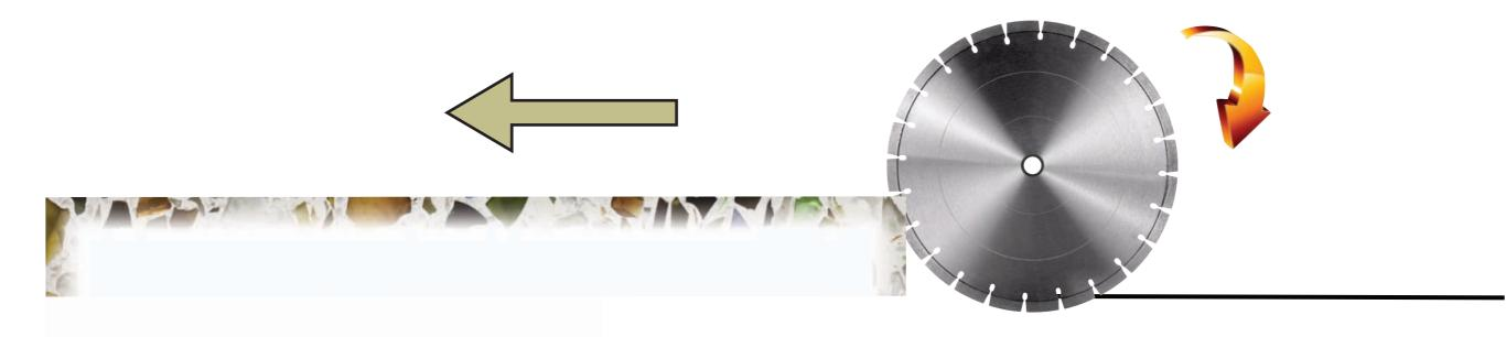
• Cut the approximately 3/8 deeper than the slab with the diamond segments running upwards into the slab (i.e. - return stroke on the bridge saw). This pass should be slower than the first pass. Always use water.
