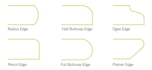
Glass segregation in some edge profiles may be pronounced. This can be addressed using a full bullnose, radius or platner edge.
