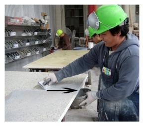
6. Scrape excess slurry into the mixing bowl. Make sure the patch dries in a consistently thin layer. Areas with too much patch will appear discolored and will require reworking.
